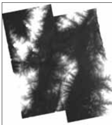
Radargrammetry & stereoscopic interpretation: from StripMap data pairs to DTM
