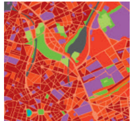
Subset of a landcover map: City Center of Brussels, Belgium; based on a TerraSAR-X acquisition with a 3m ground resolution (2008).
